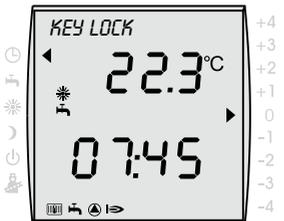
If the display shows *KEY LOCK*, then the key lock is activated.
