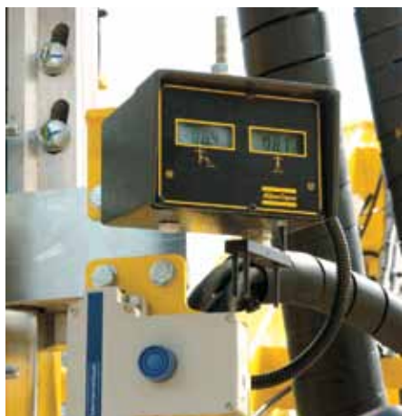
Feed mounted angle instrument.
