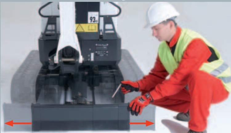
The E08 and E10 are both equipped with expandable undercarriage and blade as standard. There is no need to remove and reinstall the blade extensions.
